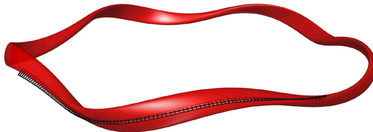
FIG. 6: (Color online) 3D visualization of the \alpha = 0 flux tube domain in real space superimposed on the flux surface
