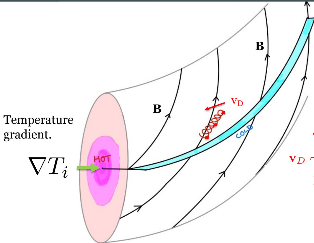
Toroidal ion drift
