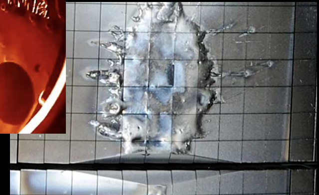
Melting caused by a runaway electron beam on JET ( https://www.iter.org/newsline/-/2234 )
