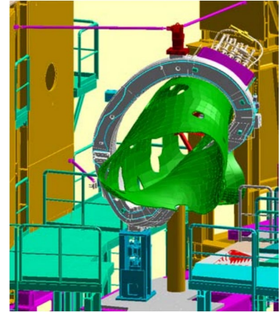
Fig. 6: Alignment of a single coil in first assembly step (CAD-drawing). Coil is fixed on a foot column in the right position. With both upper and one horizontal (left side) bar the coil is aligned to nominal position.
