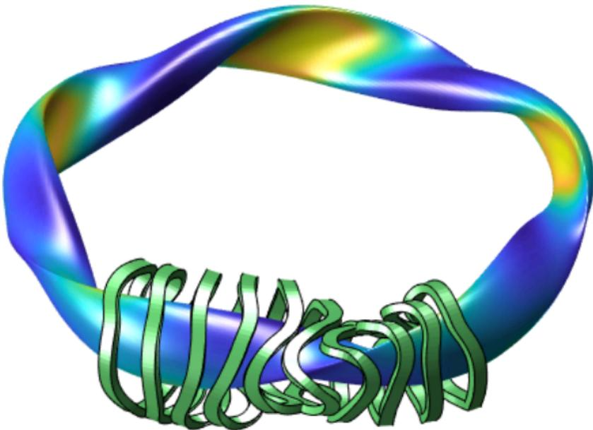
Last closed magnetic surface of the W7-X configuration
