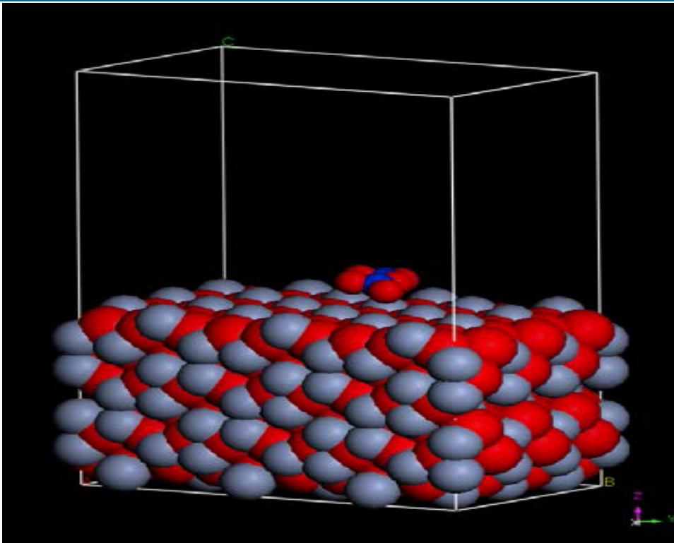
**Figure 11.** Input schematic of  $\text{N}_2\text{O}_5$  on  $\text{Cr}_2\text{O}_3$  surface.
