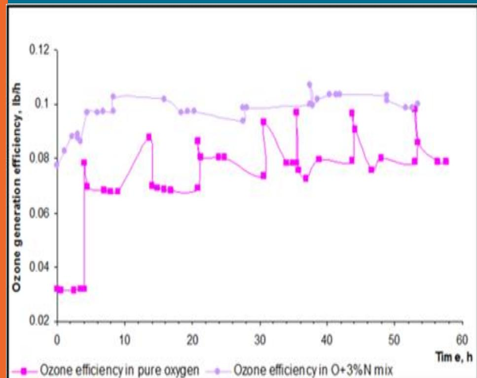
**Figure 6.** Plot of ozone production as a function of time with and without  $\text{N}_2$ .
