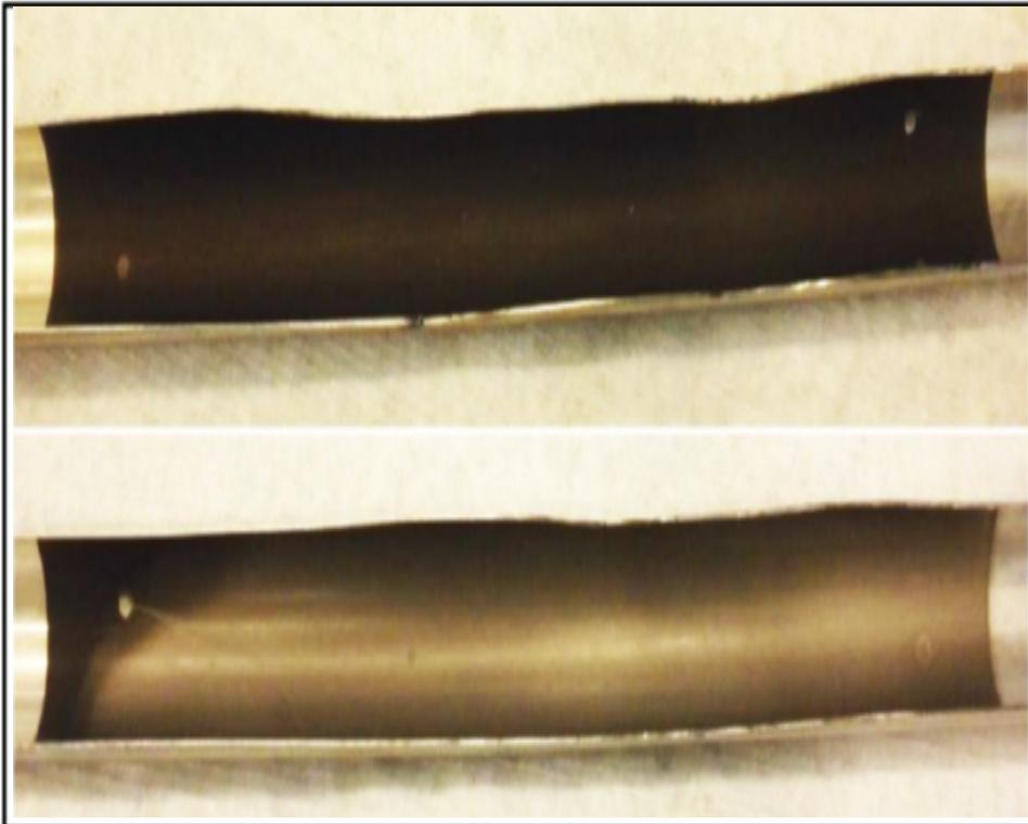
**Figure 9.** Photograph of the discharge tube when operated without N<sub>2</sub> (top) and with 2.3% N<sub>2</sub> (bottom).
