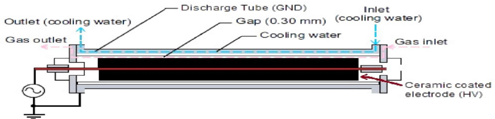
Fig. 4. Configuration of the ozone generator.
