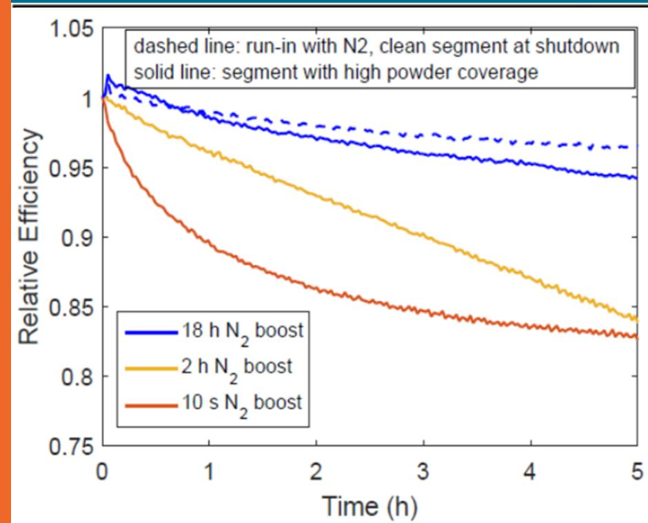
**Figure 8.** Time dependent evolution of ozone generation efficiency after shutdown of N<sub>2</sub> supply. During the experiments illustrated with solid lines, the high voltage electrode was already covered in a powder because of prior N<sub>2</sub>-free operation. The dashed line corresponds to N<sub>2</sub> shutdown initiated with no prior N<sub>2</sub>-free operation, i.e. a relatively powder-free electrode.
