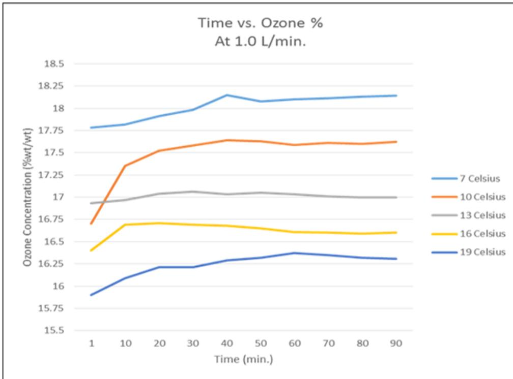
Figure 5. Water-cooled reactor with pure  $O_2$  at 1.1 bar pressure and constant input power of 160 Watts.
