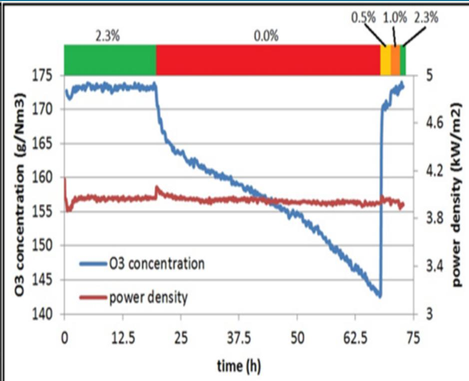
**Figure 7.** Plot of ozone production efficiency as a function of  $\text{N}_2$  inclusion at constant power density and temperature
