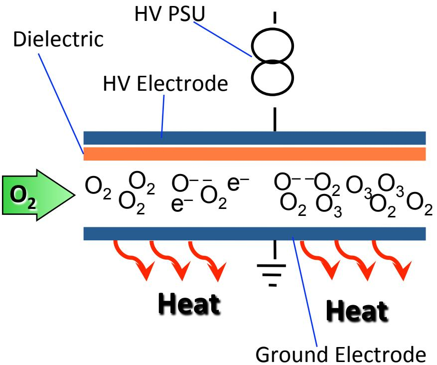
Figure 4. Ozone generator diagram.
