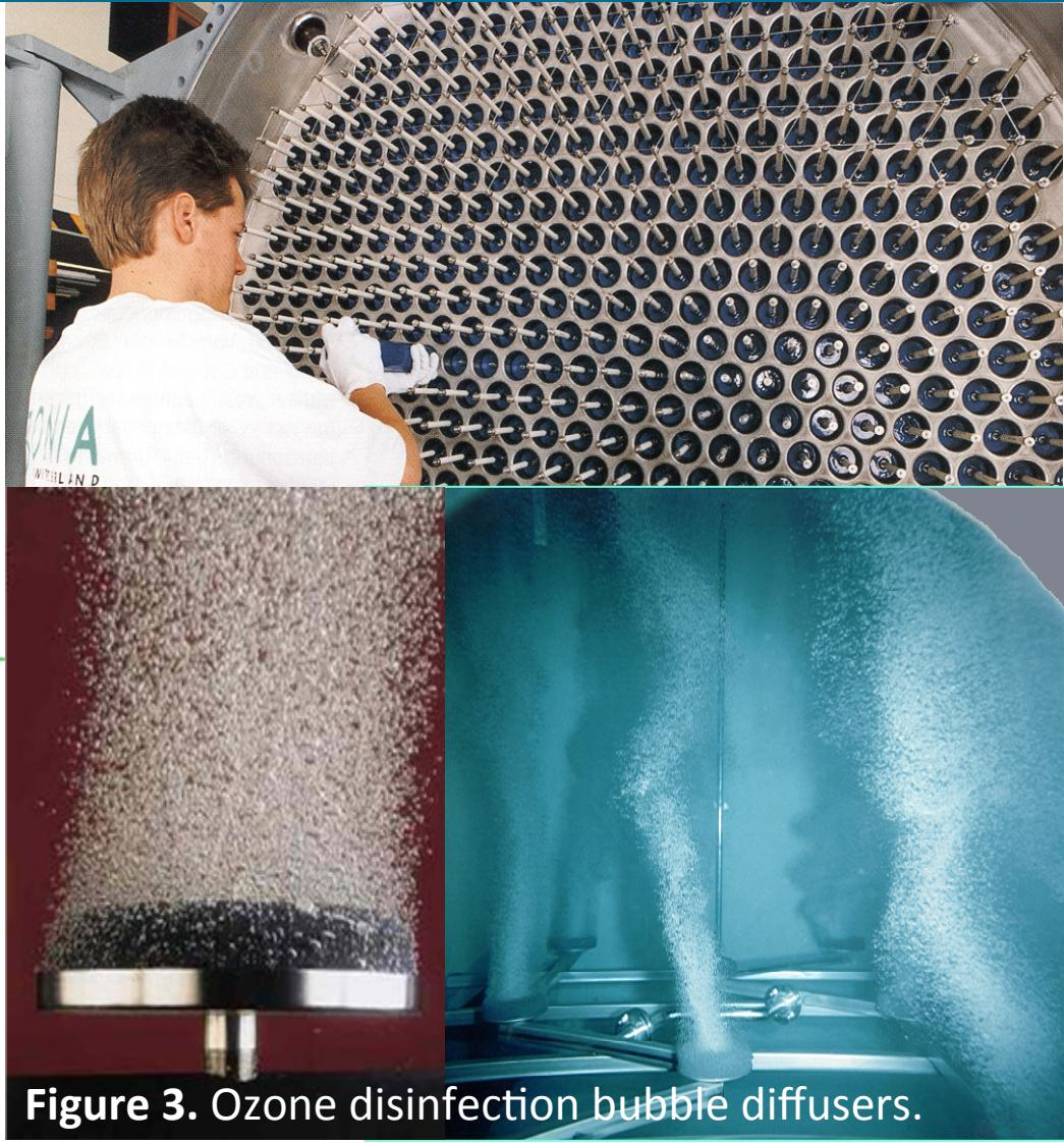
**Figure 3.** Ozone disinfection bubble diffusers.
