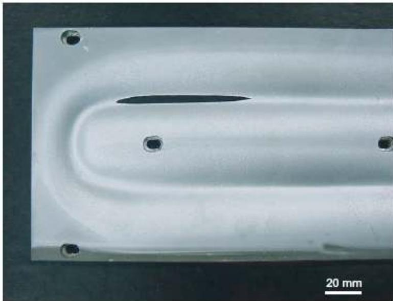
Eroded rectangular target sputtered with a conventional magnetron cathode, showing faster etching in the upper left corner area.
